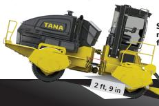
Safe design without belly pans: no debris accumulation to cause any fire hazards.
