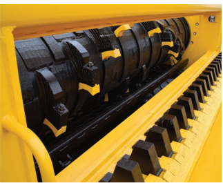
Hardface weld surfacing to extend the life of the rotor
